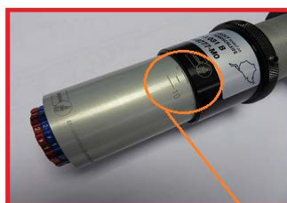
Upright height Adjuster 0mm (-10mm to +10mm)
