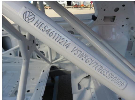
V.I.N. (Vehicle Identification Number) is welded on the roll cage
