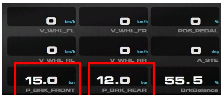
Set rear brake proportion valve on position on the desired position (standard position: 3)
