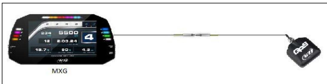
Data-logger standard connection scheme (car delivery)
