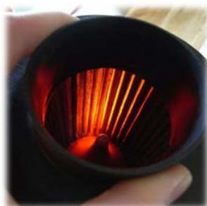
8. Once it is evenly coated, leave it stand for 30 minutes. Carefully pat the excess off the filter with paper towels.
